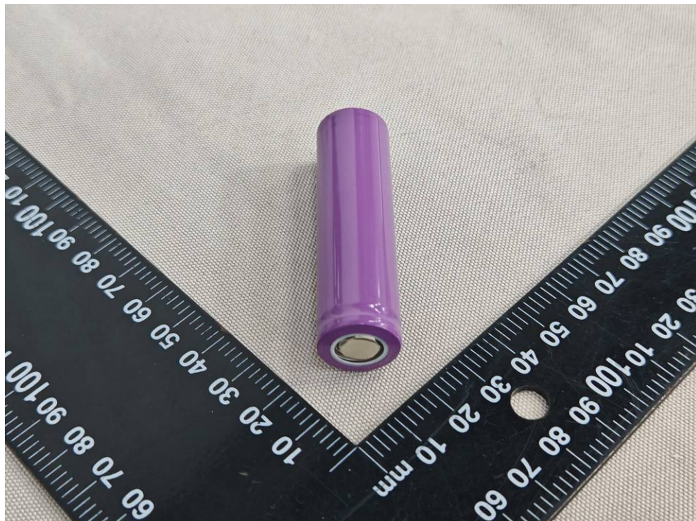
Figure 16 Side view of cell (Model: IMR18650-1200mAh)
