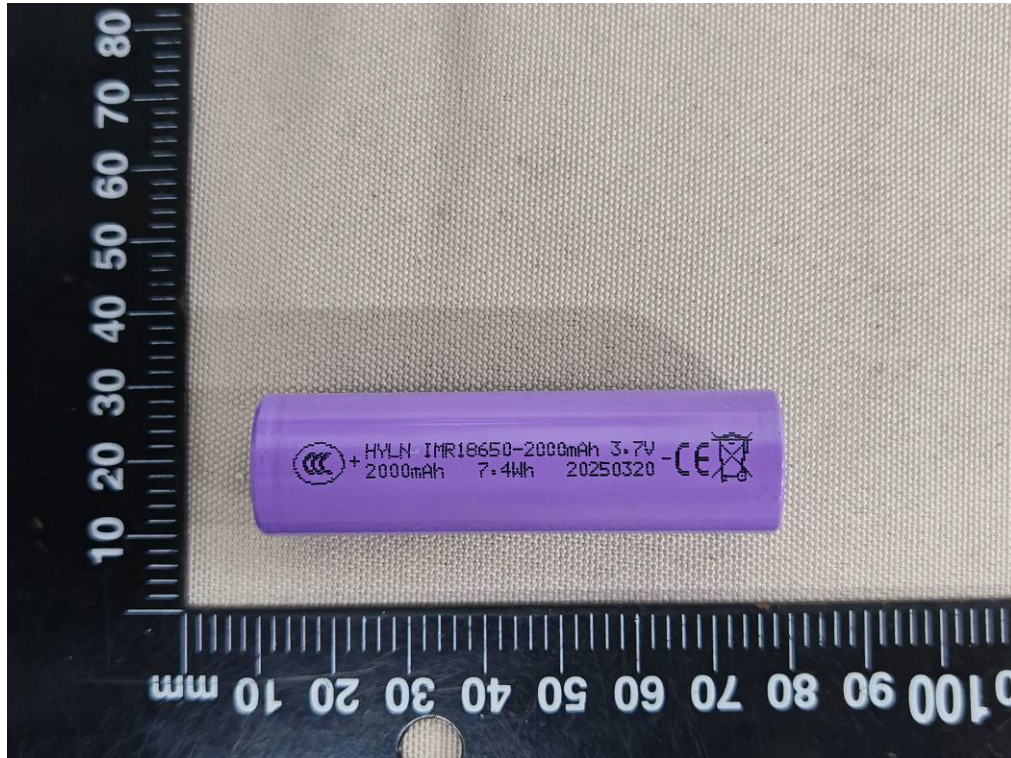
Figure 9 Front view of cell (Model: IMR18650-2000mAh)
