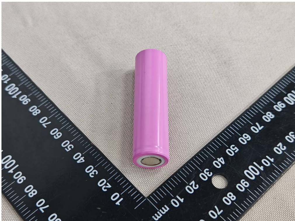
Figure 8 Side view of cell (Model: IMR18650-2200mAh)
