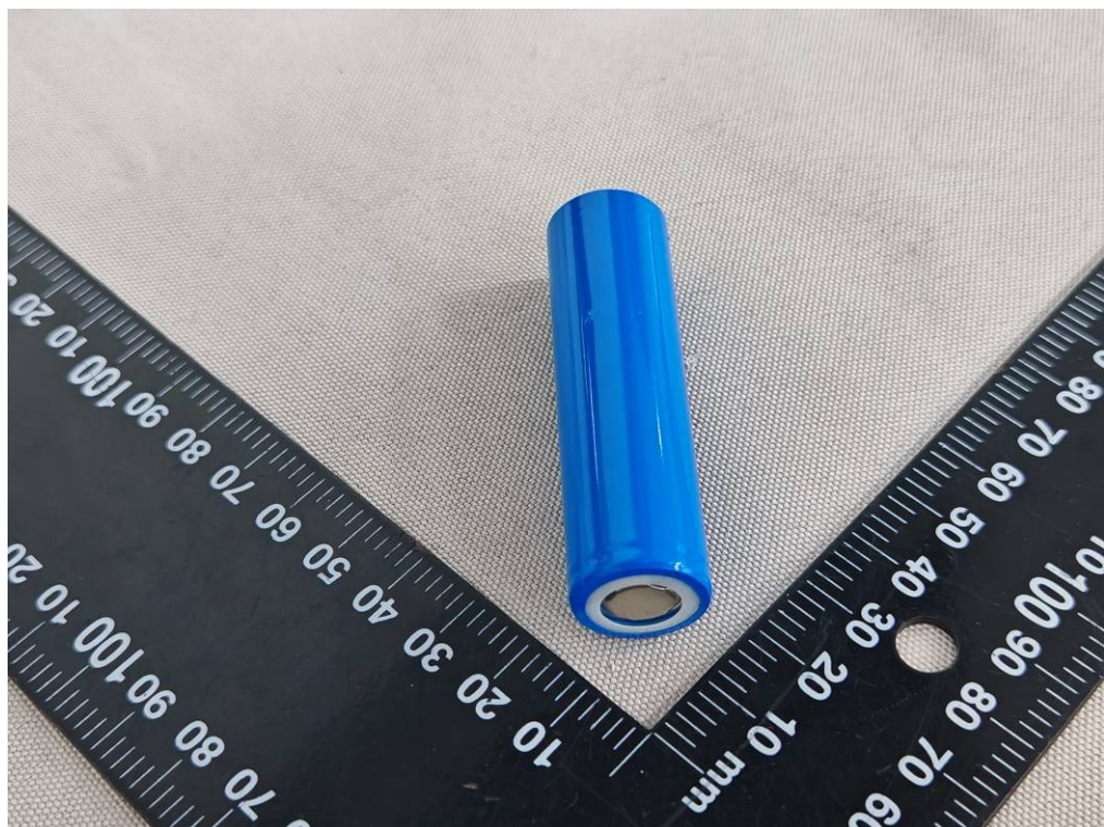
Figure 12 Side view of cell (Model: IMR18650-1800mAh)
