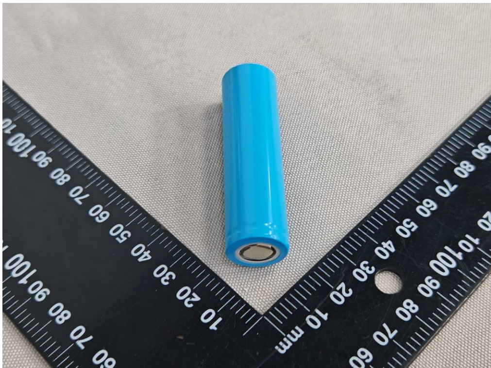
Figure 14 Side view of cell (Model: IMR18650-1500mAh)
