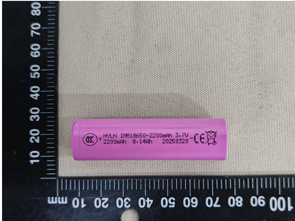
Figure 7 Front view of cell (Model: IMR18650-2200mAh)
