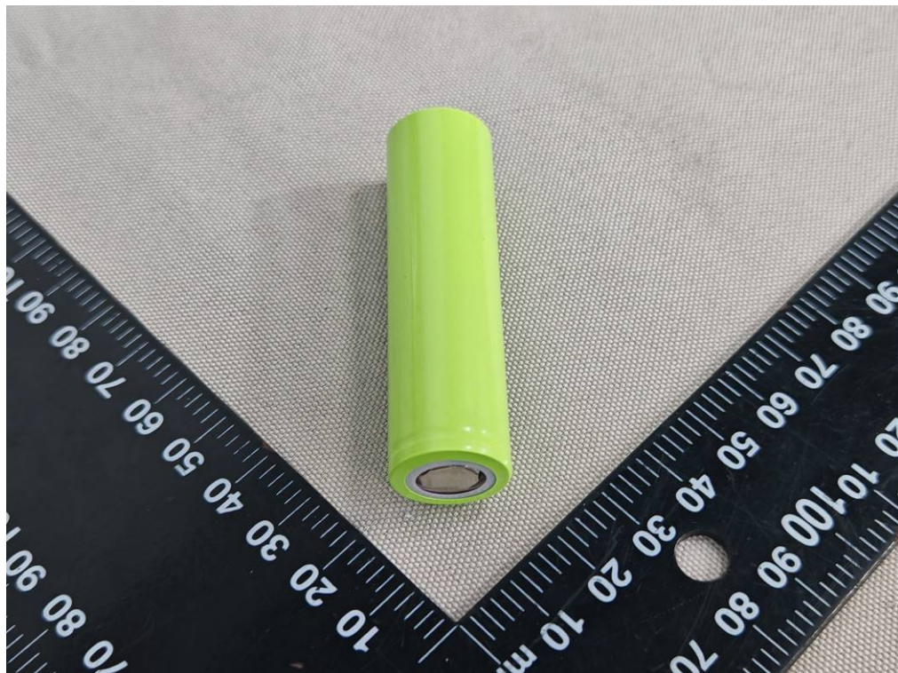
Figure 6 Side view of cell (Model: IMR18650-2500mAh)
