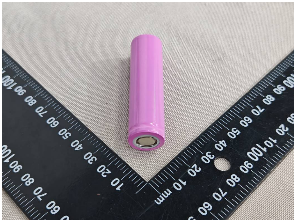
Figure 18 Side view of cell (Model: IMR18650-800mAh)
