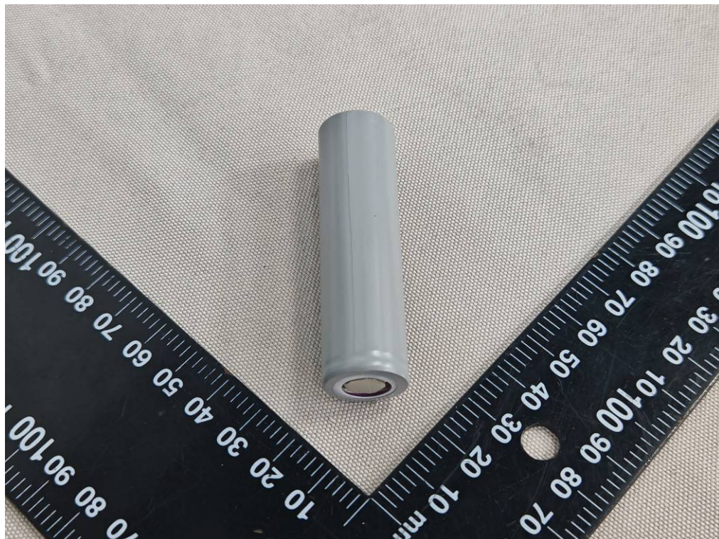
Figure 4 Side view of cell (Model: IMR18650-2600mAh)
