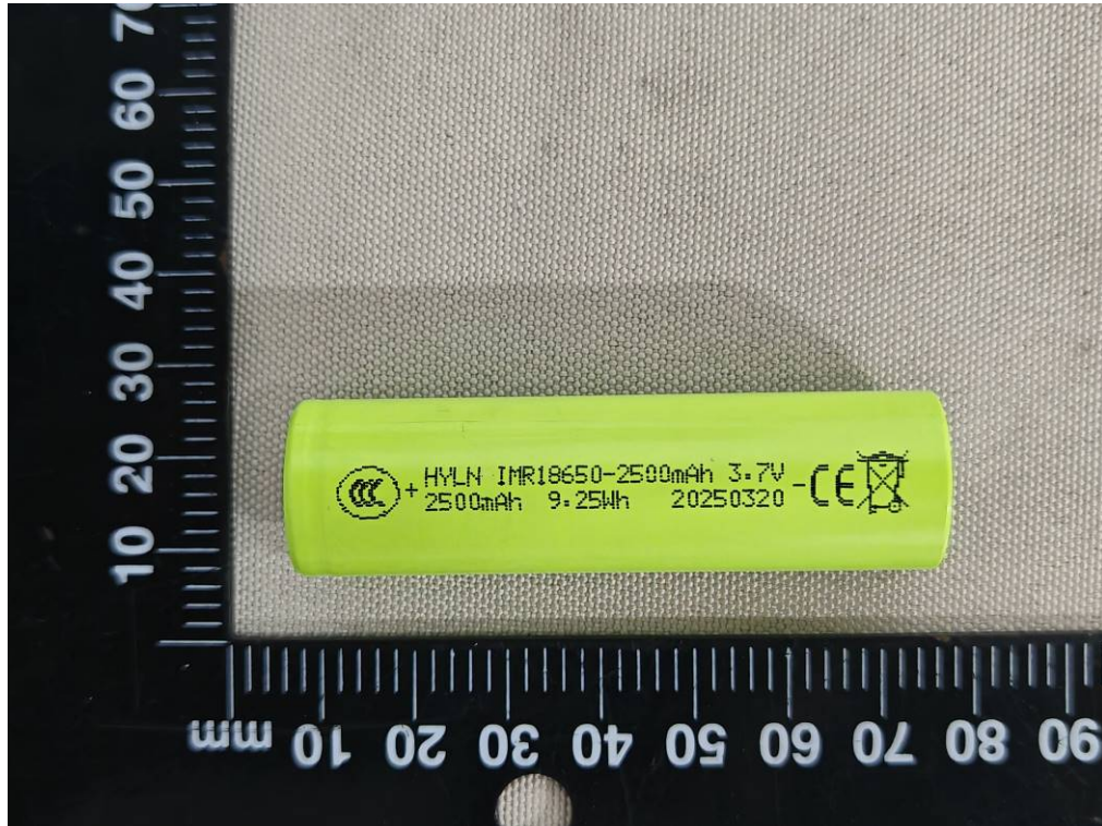
Figure 5 Front view of cell (Model: IMR18650-2500mAh)
