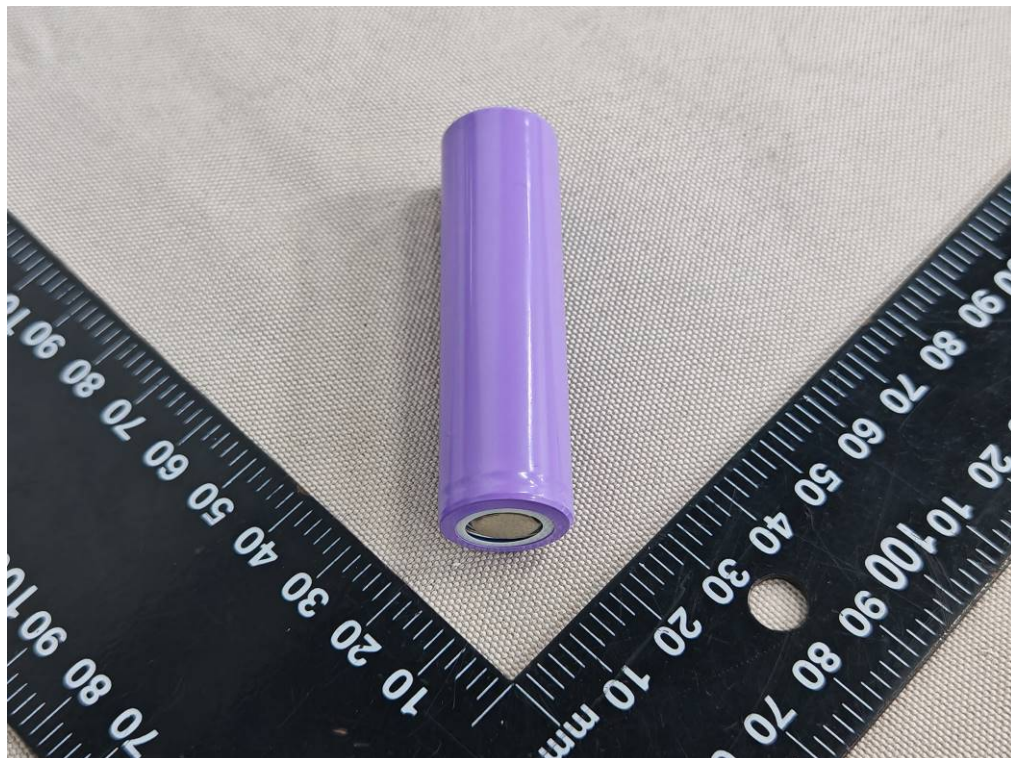
Figure 10 Side view of cell (Model: IMR18650-2000mAh)
