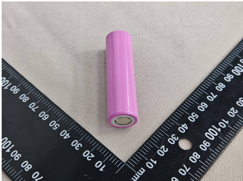
Figure 2 Side view of cell (Model: IMR18650-3000mAh)
