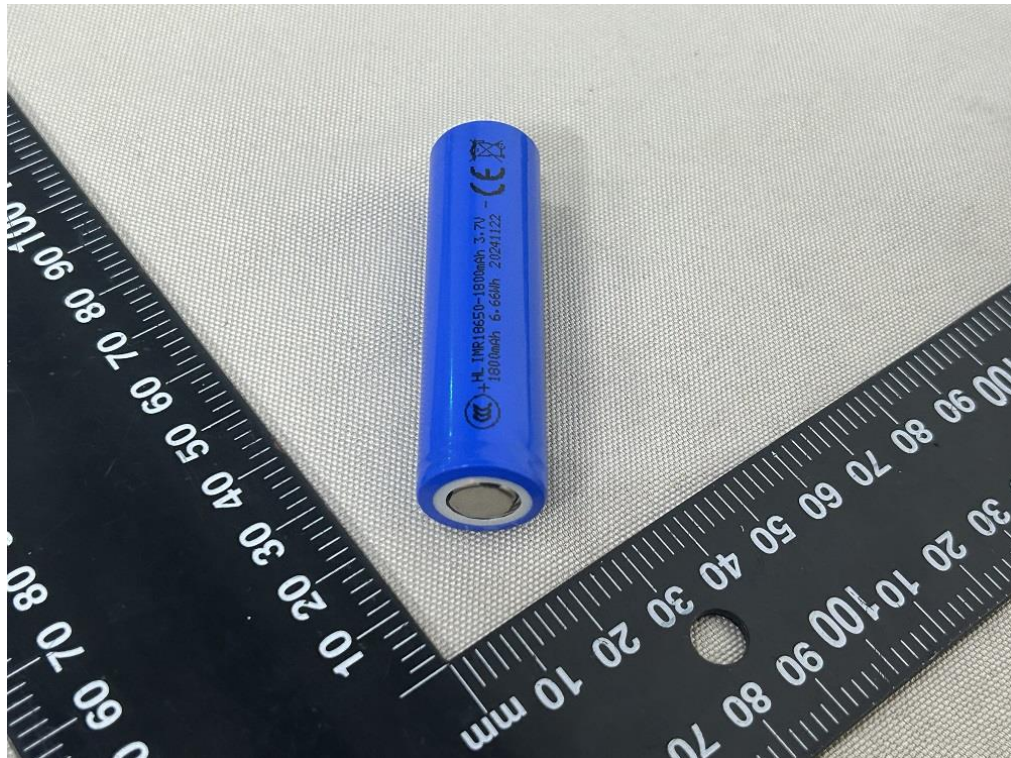
Figure 28 Side view of cell (Model: IMR18650-1800mAh) (marking 2)
