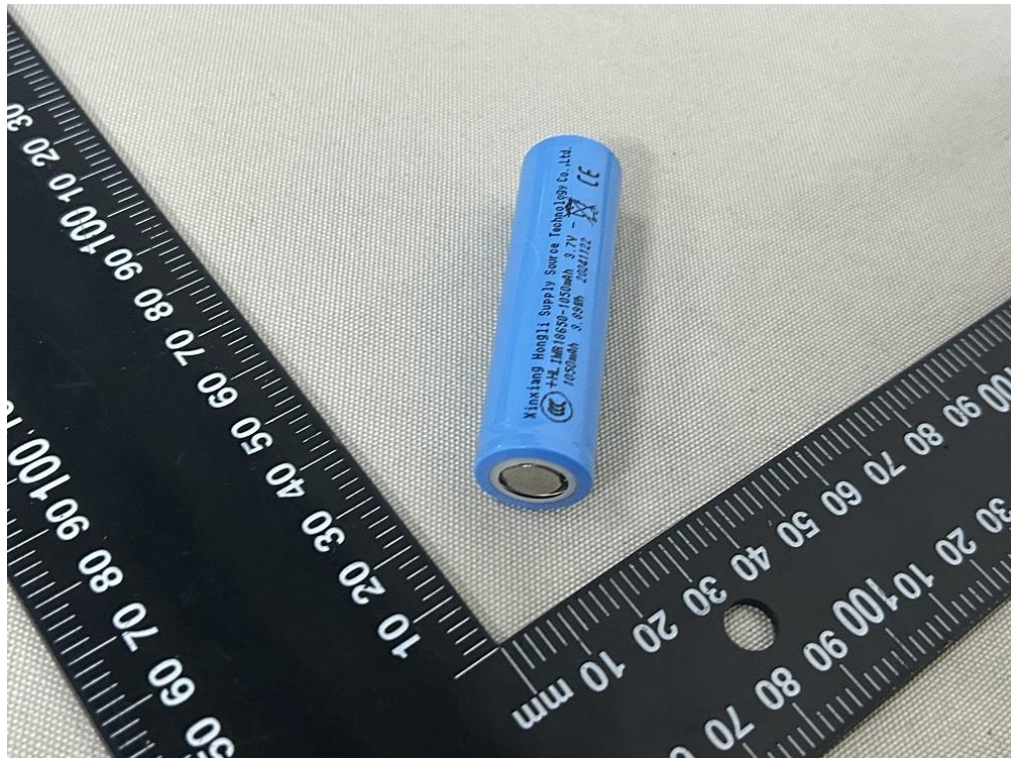
Figure 14 Side view of cell (Model: IMR18650-1050mAh) (marking 1)
