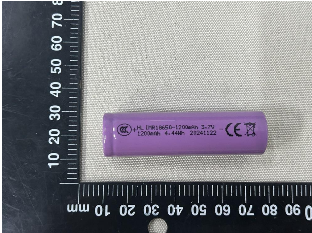
Figure 19 Front view of cell (Model: IMR18650-1200mAh) (marking 2)
