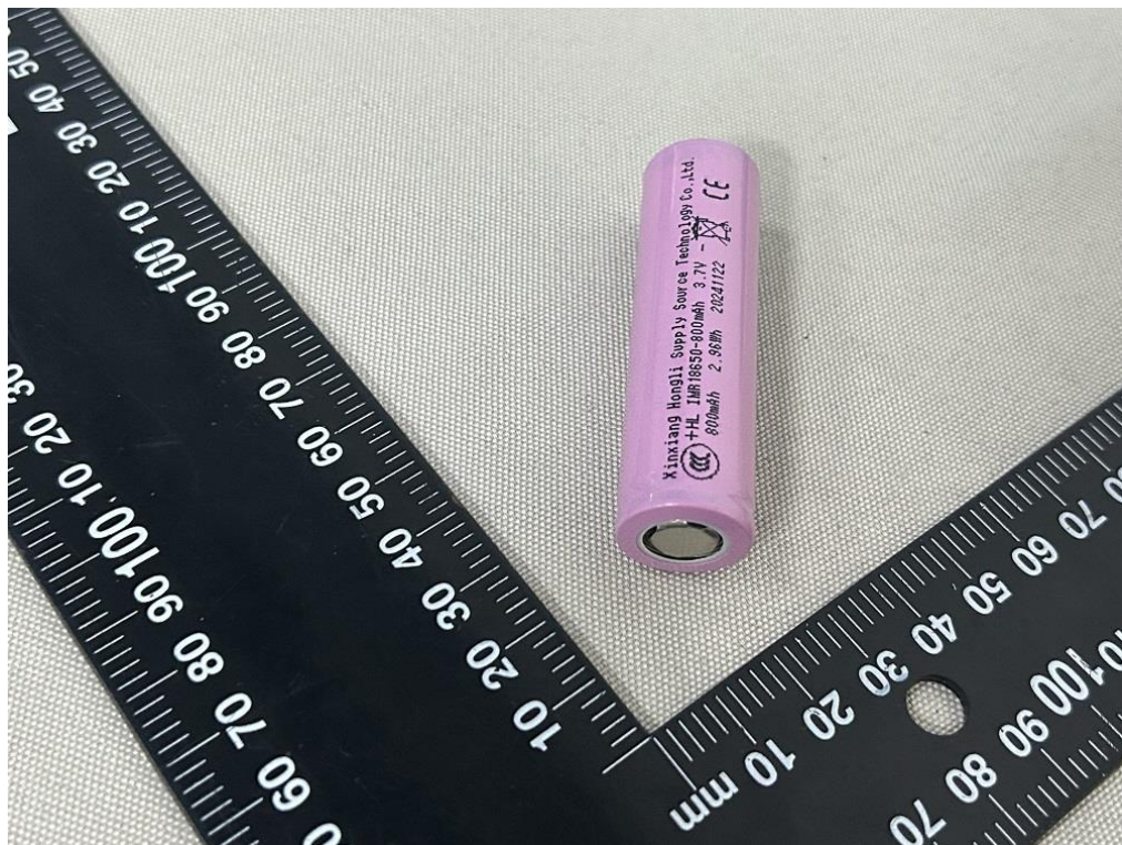
Figure 10 Side view of cell (Model: IMR18650-800mAh) (marking 1)
