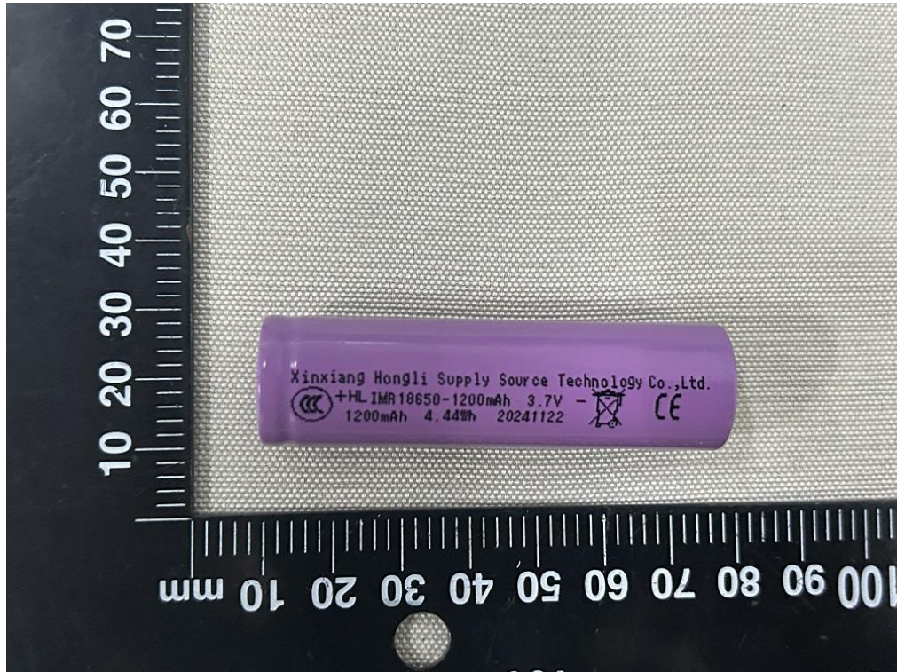
Figure 17 Front view of cell (Model: IMR18650-1200mAh) (marking 1)
