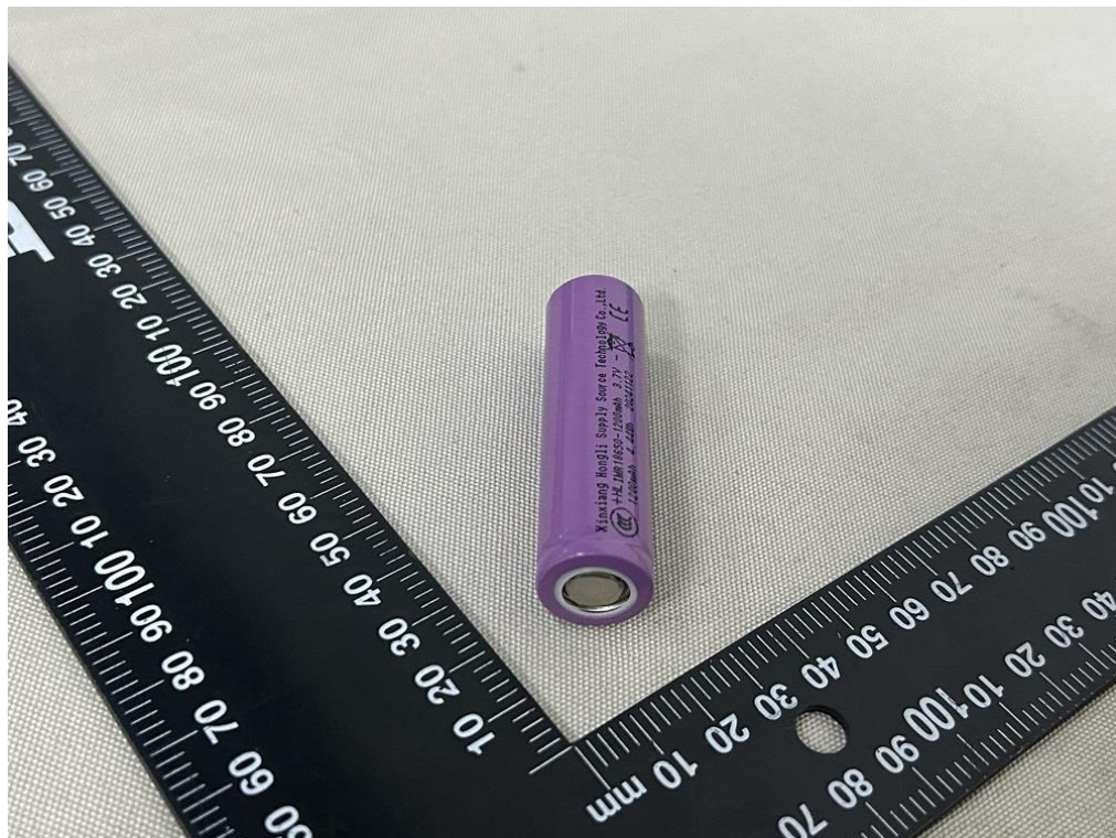
Figure 18 Side view of cell (Model: IMR18650-1200mAh) (marking 1)
