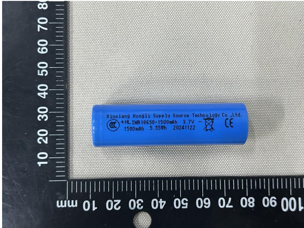
Figure 21 Front view of cell (Model: IMR18650-1500mAh) (marking 1)
