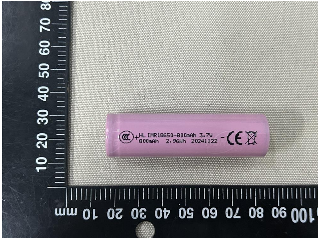
Figure 11 Front view of cell (Model: IMR18650-800mAh) (marking 2)
