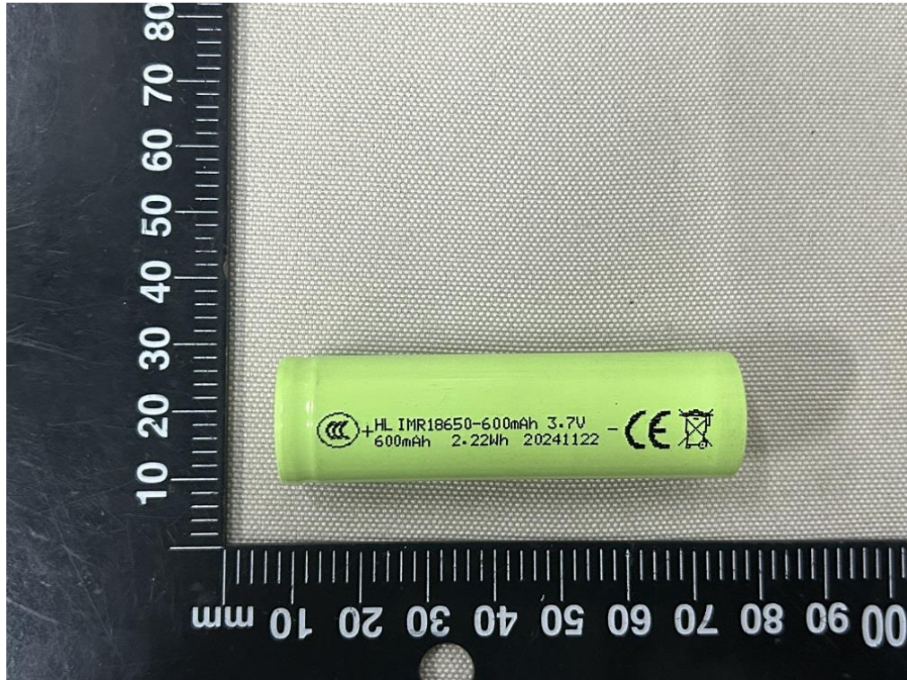
Figure 3 Front view of cell (Model: IMR18650-600mAh) (marking 2)
