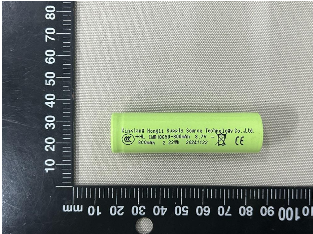
Figure 1 Front view of cell (Model: IMR18650-600mAh) (marking 1)
