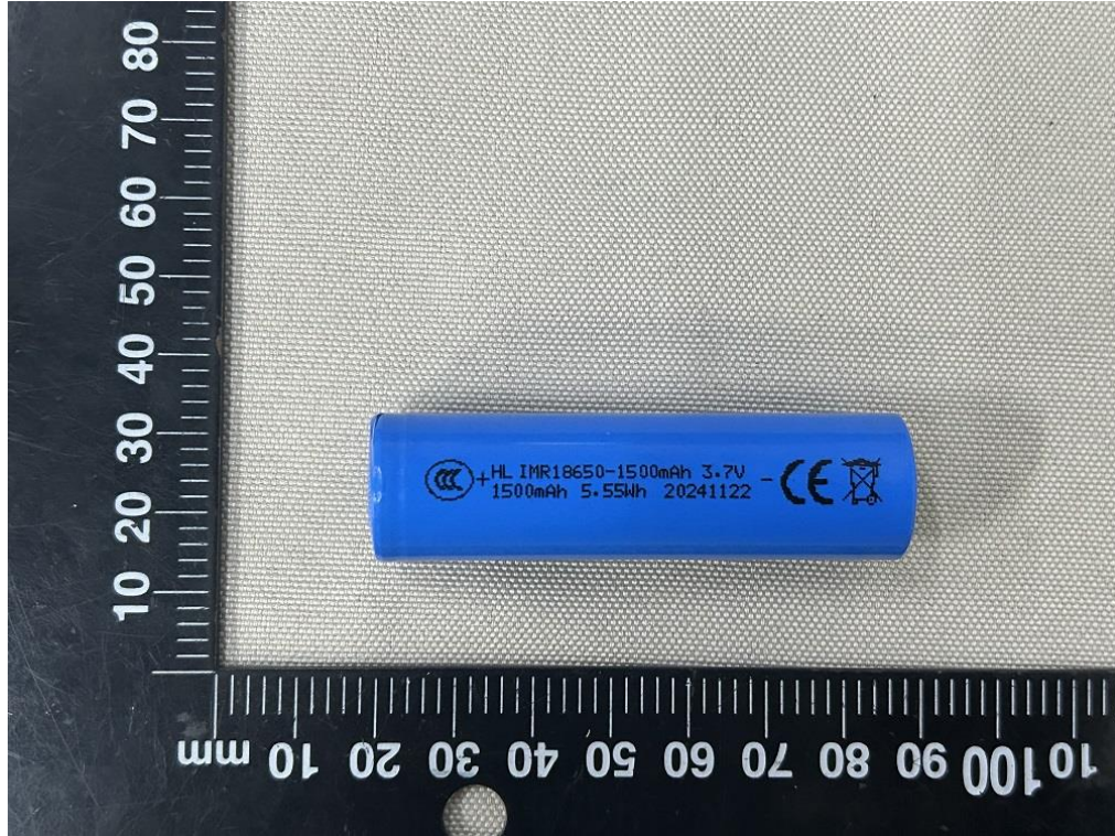
Figure 23 Front view of cell (Model: IMR18650-1500mAh) (marking 2)
