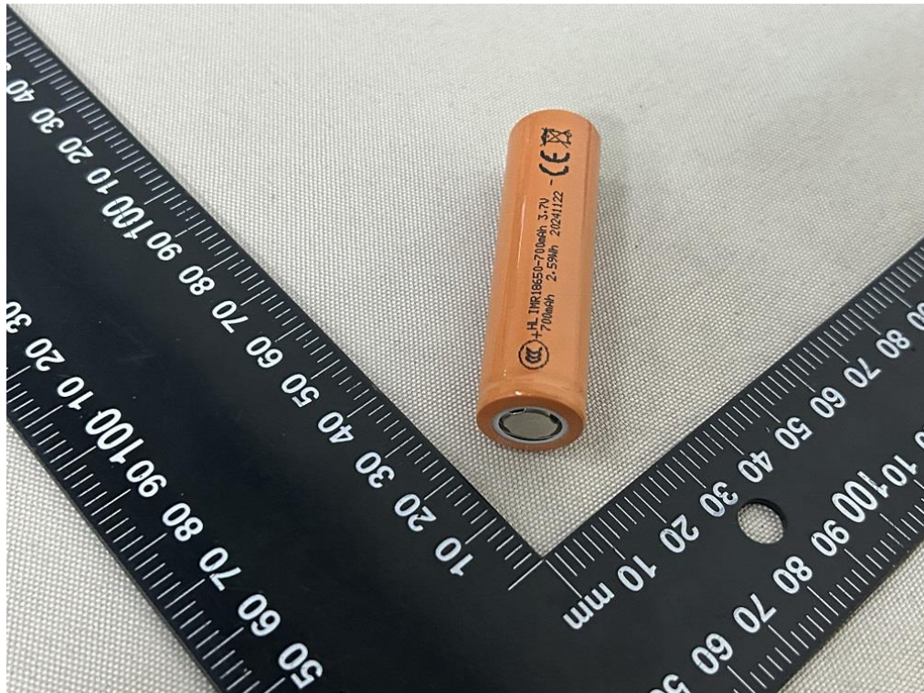
Figure 8 Side view of cell (Model: IMR18650-700mAh) (marking 2)
