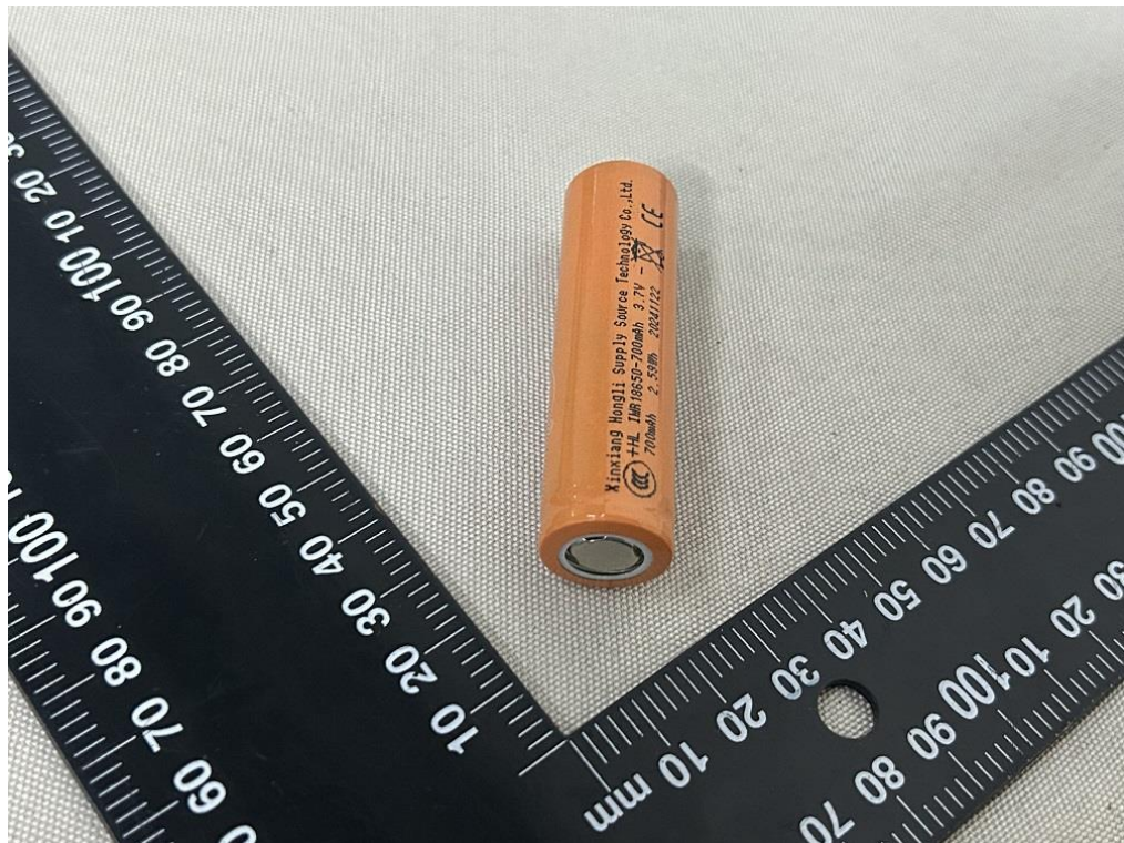
Figure 6 Side view of cell (Model: IMR18650-700mAh) (marking 1)
