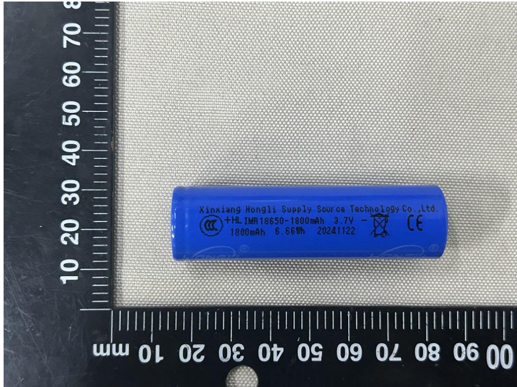
Figure 25 Front view of cell (Model: IMR18650-1800mAh) (marking 1)
