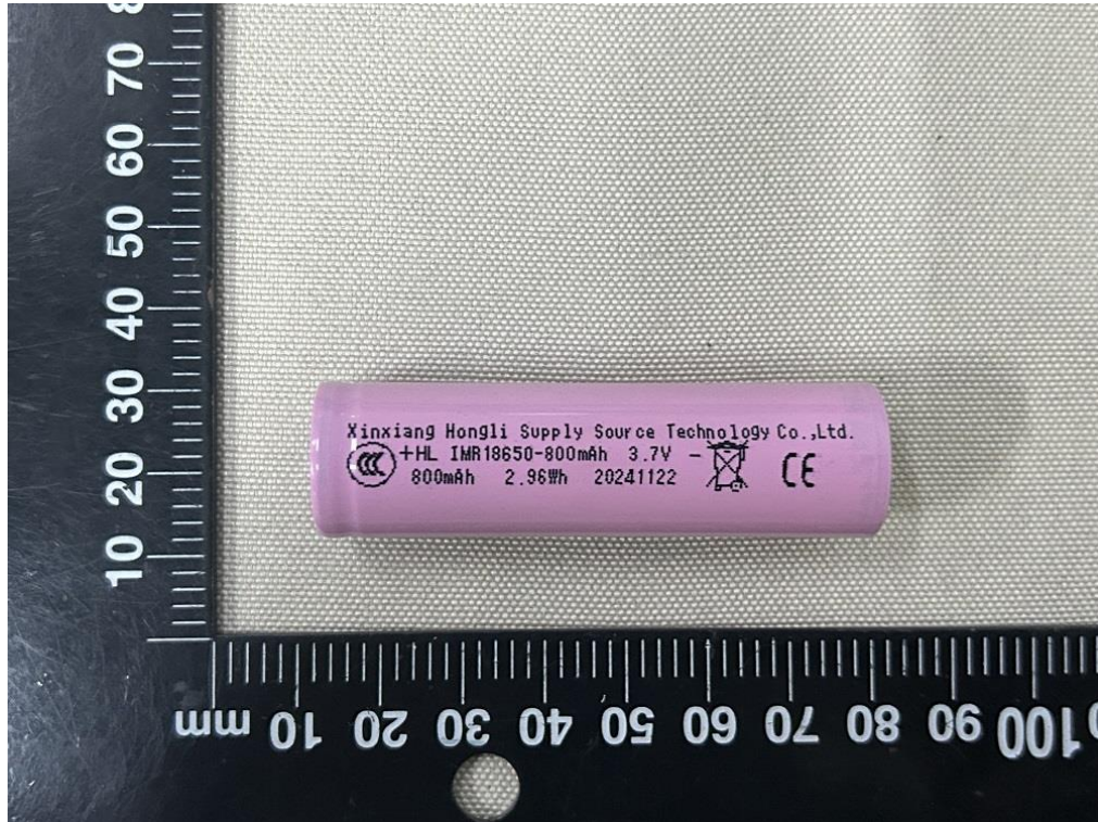
Figure 9 Front view of cell (Model: IMR18650-800mAh) (marking 1)
