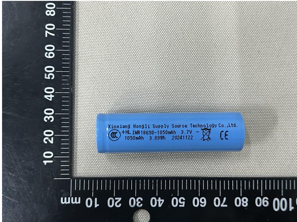
Figure 13 Front view of cell (Model: IMR18650-1050mAh) (marking 1)
