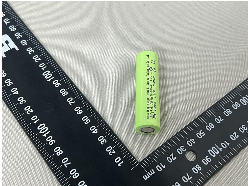
Figure 2 Side view of cell (Model: IMR18650-600mAh) (marking 1)
