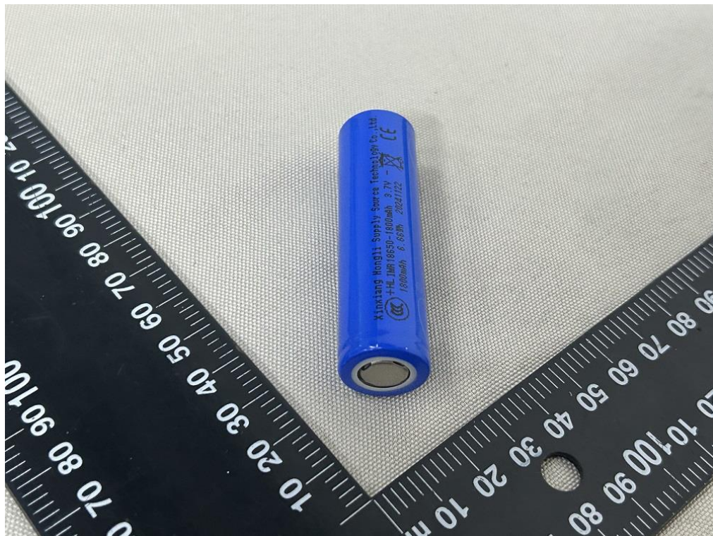
Figure 26 Side view of cell (Model: IMR18650-1800mAh) (marking 1)
