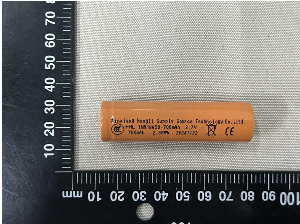
Figure 5 Front view of cell (Model: IMR18650-700mAh) (marking 1)
