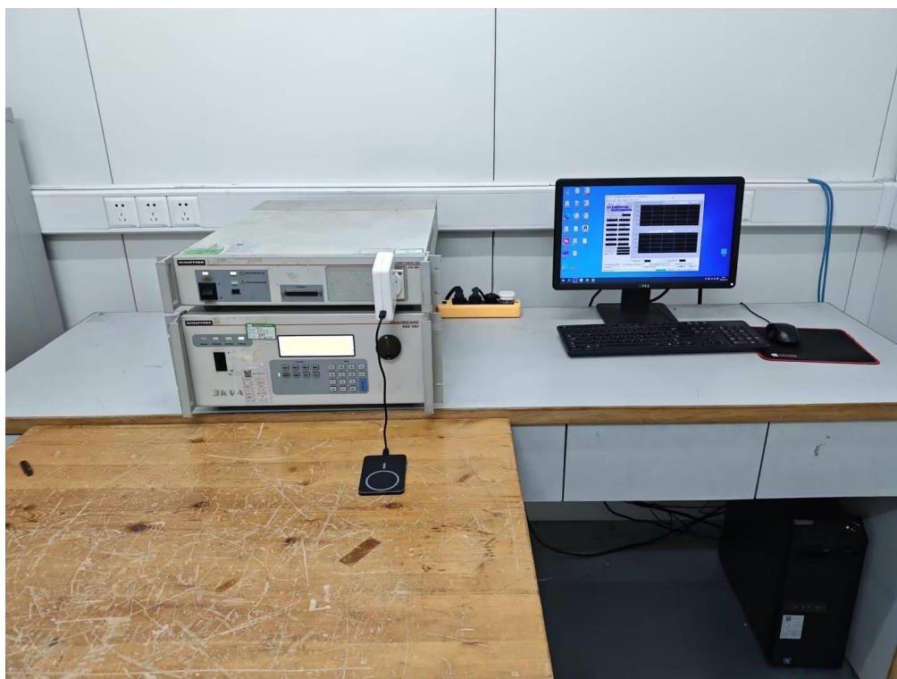
Harmonic current emissions & Voltage fluctuations and flicker
