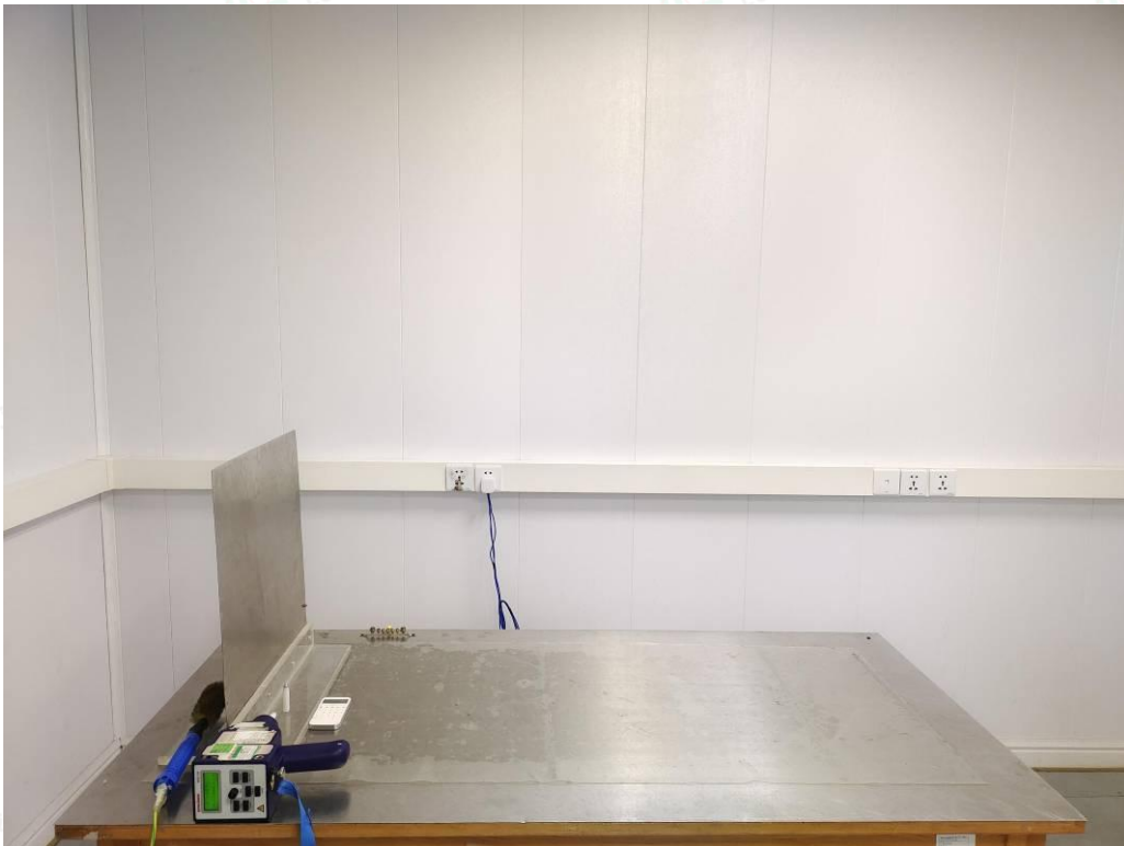
Test Setup Photo of Electrostatic Discharge Test
