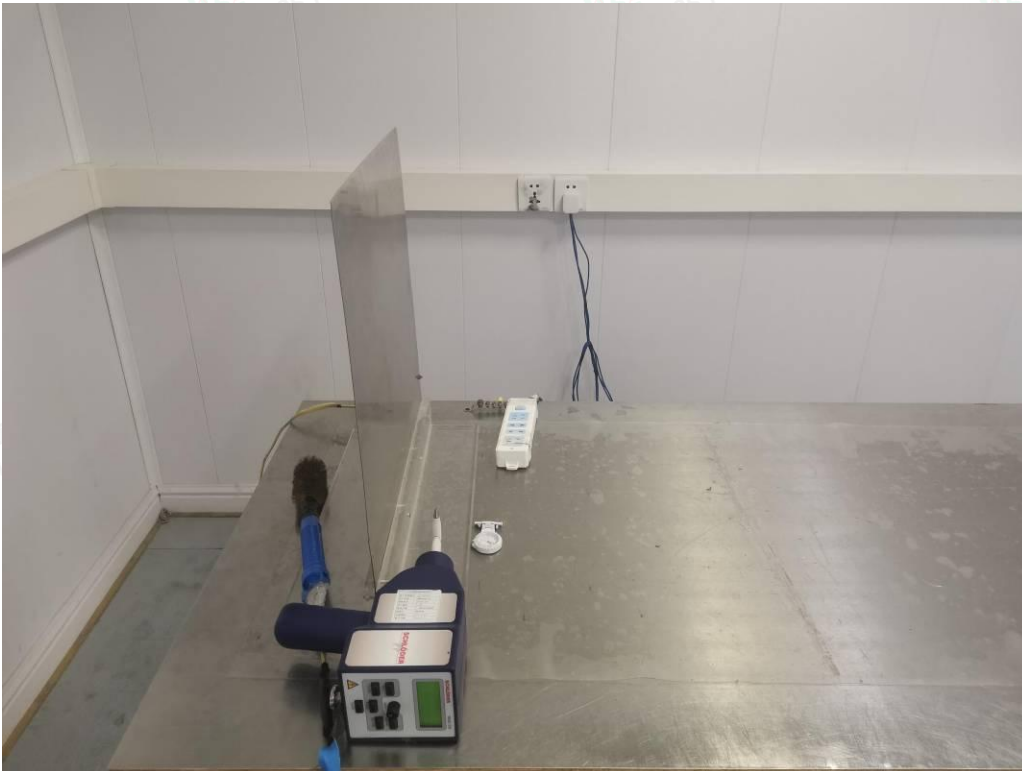
Test Setup Photo of Electrostatic Discharge Test
