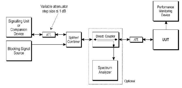
Figure 6: Test Set-up for receiver blocking
