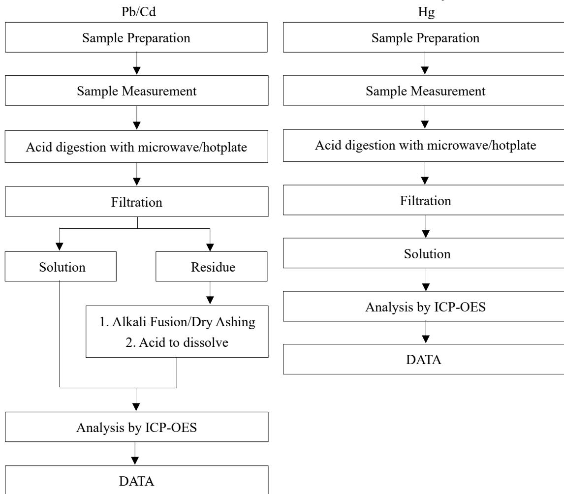
These sample were dissolved totally by pre-conditioning method according to above flow chart
