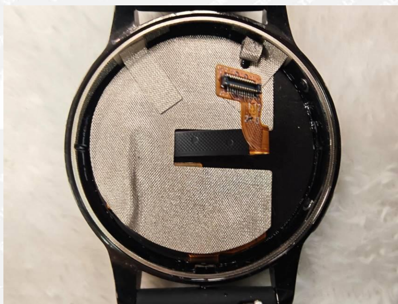
Photo 10 -- After the test of IPX7
