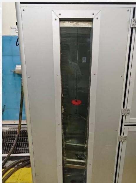
Photo 7 -- During the test of IPX7
