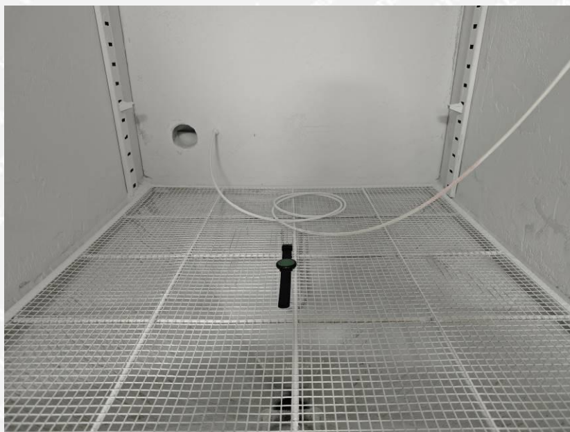
Photo 3 -- During the test of IP6X
