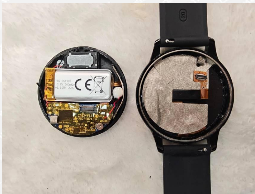
Photo 8 -- After the test of IPX7
