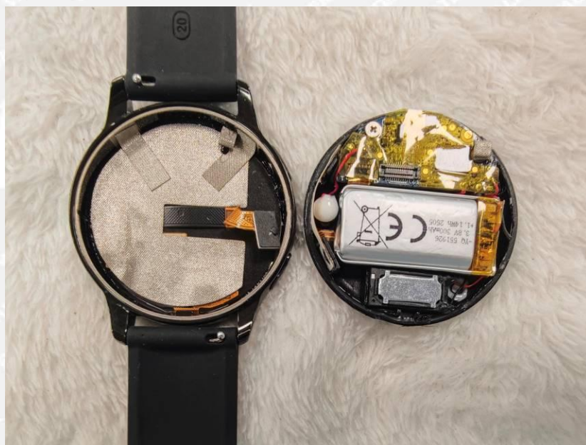
Photo 4 -- After the test of IP6X
