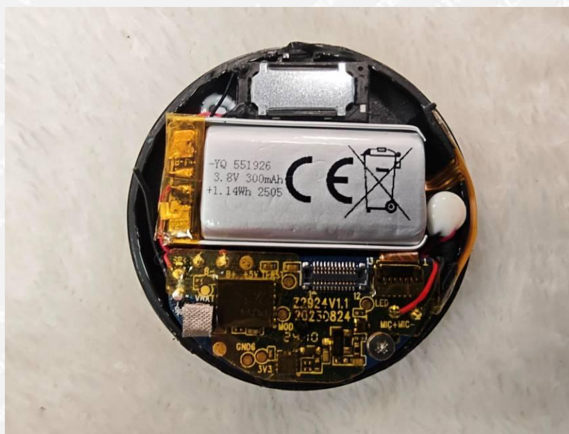
Photo 9 -- After the test of IPX7
