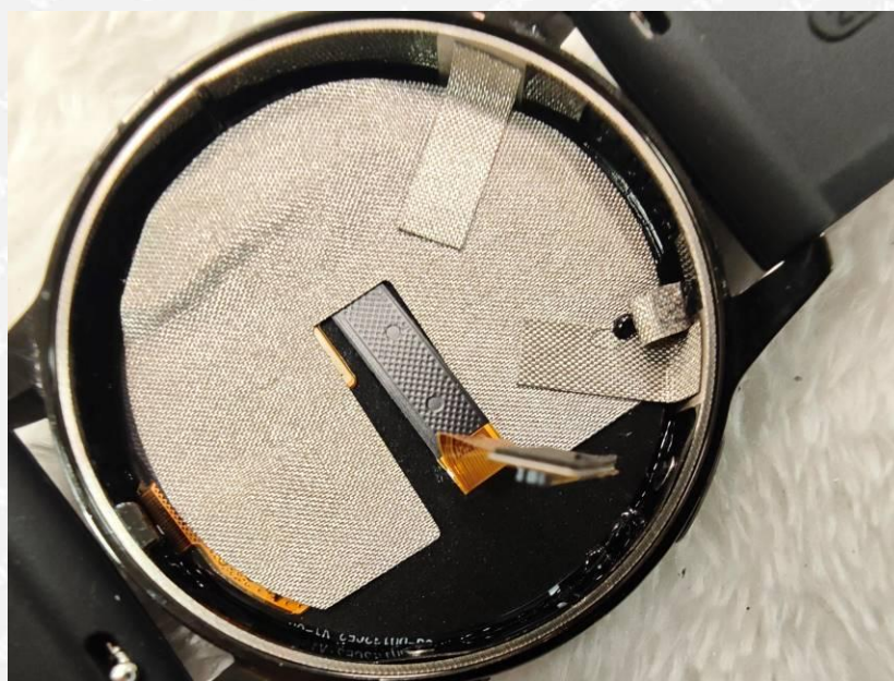
Photo 5 -- After the test of IP6X
